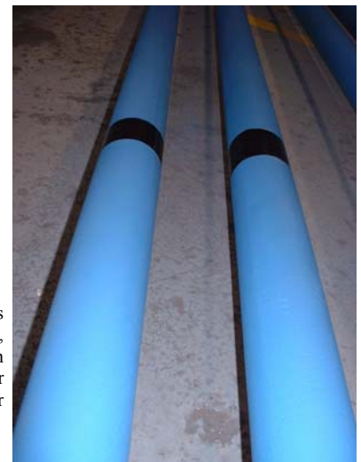
Applied for aggressive gas and downwell service, CORROLON III™ is seen here on 2 5/8” J55 Tubular Pipes (32 Ft. Randoms) for chemical environments.
